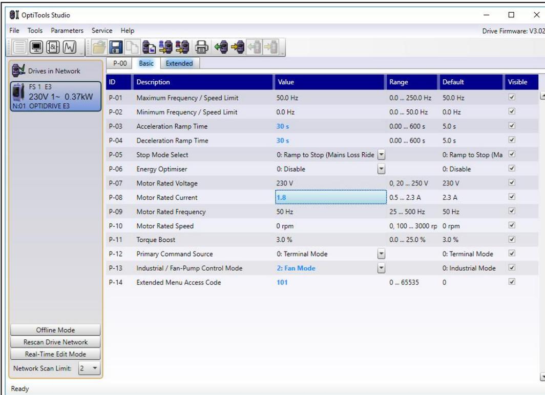
Make any changes to the parameter set as required. Changes from Invertek factory default settings are highlighted in blue.
